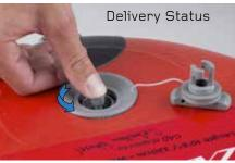
Make sure that the valve on the Fanatic Fly Air is in the outer position. The valve must be released for inflation. To release the valve, push lightly downwards and twist to the left or right (see picture). The valve is now in the upper position.
